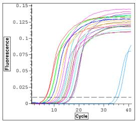
The dotted line in the graph represents the "threshold" above which the product of a reaction is deemed to be significant. The Cycle-Threshold ( $C_T$ ) is the numeric value for the cycle at which the product crossed the threshold. Reactions with lower  $C_T$  values contain more of the gene of interest since they took less time to amplify. In the same way, samples with a higher  $C_T$  contain less of the gene of interest.
