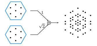
• Two lattice codewords can be recovered from their linear combination if the ratio of the coefficients is irrational.
